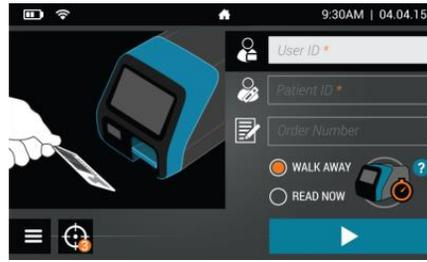
2. Input the Patient ID and/or Order # (if applicable) using the integrated barcode scanner or enter the data using the on-screen key pad.
