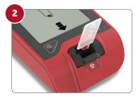
Place the microcuvette into the analyzer.
