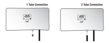
**NOTE:** Rubbing alcohol or soapy water can facilitate connections. Make sure connection is secure.
