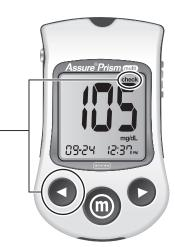
Compare the result displayed on the meter to the range printed on the test strip bottle or box of individually wrapped test strips. If the result falls within the specified range, you are ready to use the meter and test strips to test with blood.
